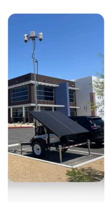
The LotGuard PRO Trailer can be fitted with up to 4 advanced PTZ IR cameras that offer a near 360 degree view and zoom in capabilities. This also allows them to view up to 200 meters in the dark, ensuring your parking lot is protected when it's most vulnerable.
